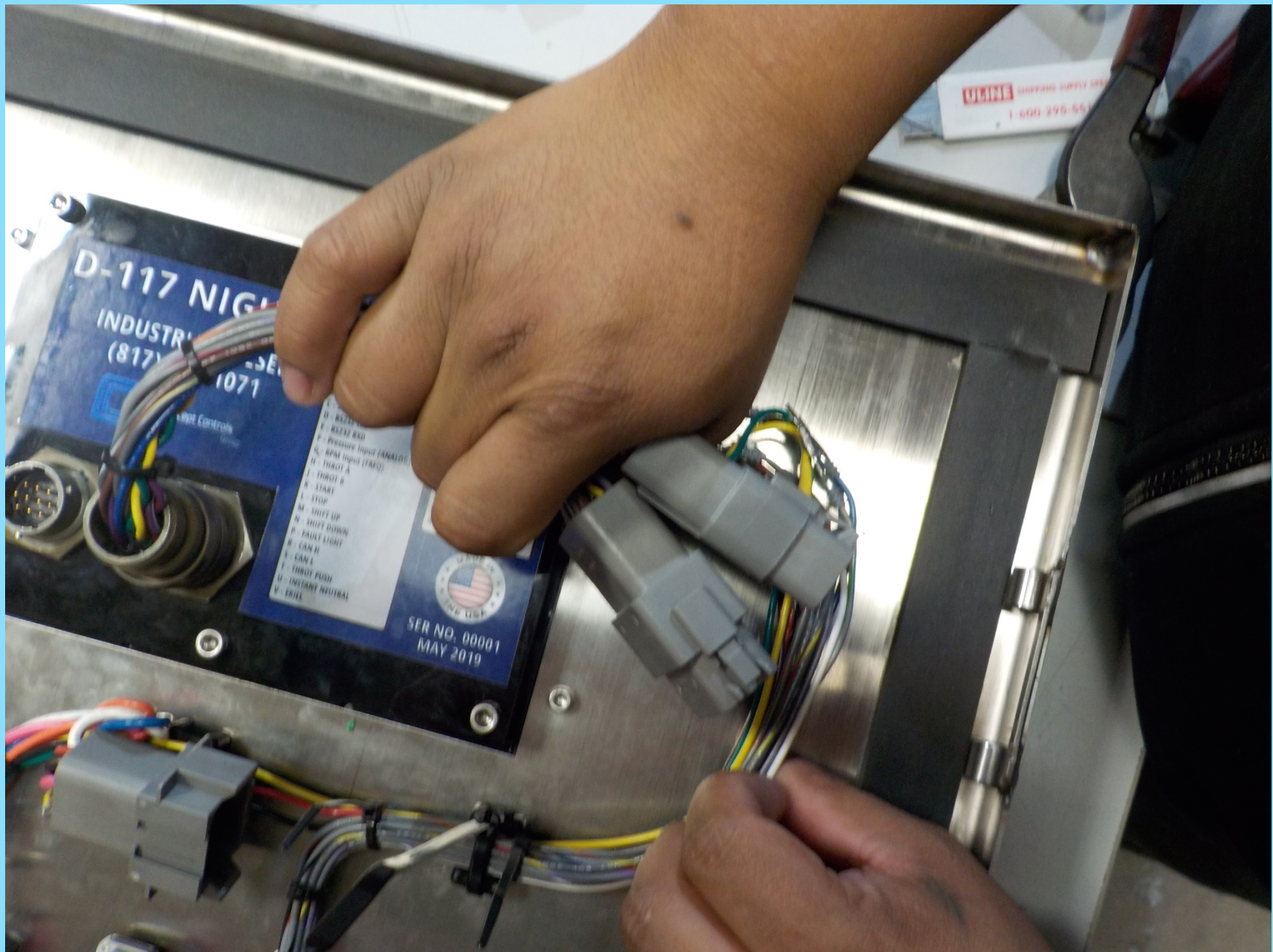
Plug the pigtail (D-117-PIGTAIL) into the back of the Display.
