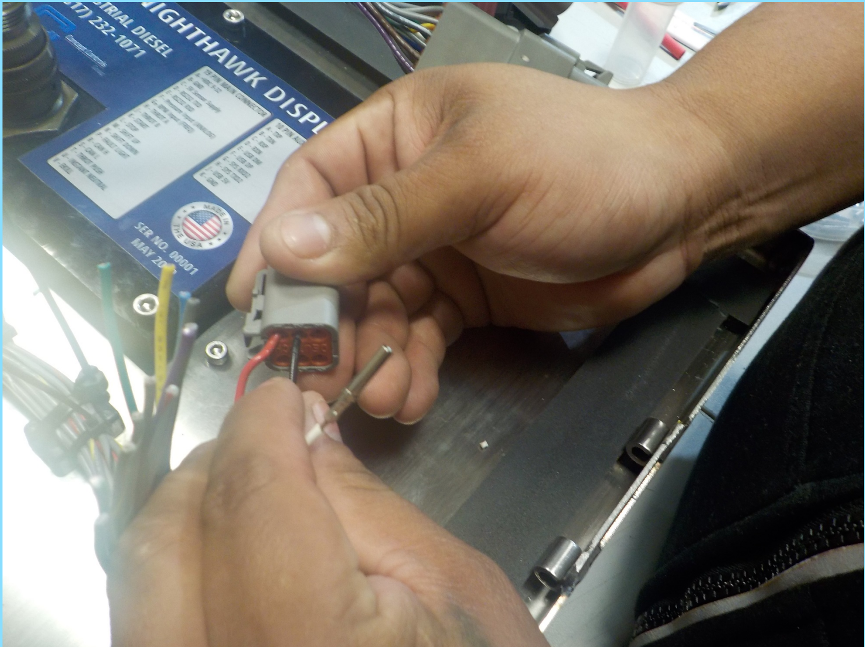
Red, Black, and White wires go to 6 socket DT Connector (DT06-6S). red-1, black-2, white-3.
